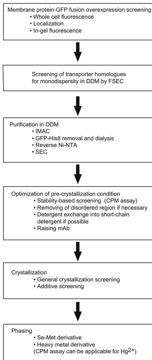
**Fig. 3.** Schematic flow diagram illustrating the steps towards crystal structures of transporters.
